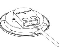
Attach the alarm by twisting clockwise into the power supply unit until it clicks. If the battery is either missing or inserted incorrectly, the smoke alarm will not be able to click into the power
