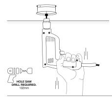
Screw recess kit base onto the ceiling. Then screw power supply unit inside the recess kit base.
