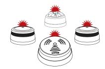
When all alarms flash the red **LED**, they are connected and can be switched out of '**Learn Mode**' and installed.
