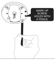
Screw the mounting base on the ceiling.
