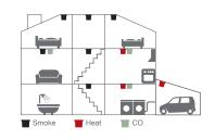
Placement: Designed for placement on ceiling (preferred) or wall. The smoke alarm should be a minimum 50cm from the wall, with a minimum of one smoke alarm per floor and a maximum distance between smoke alarms of 10 metres
