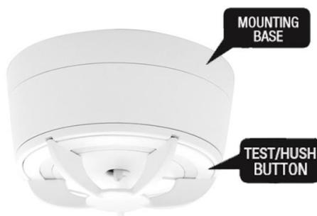
**LOW BATTERY INDICATOR:** Inside the batter chamber is a 5 Year Lithium CR123A replaceable battery. A short acoustic “beep” will sound when the battery is near its end of life. In this stage, it will continue for a maximum of 30 days. You can replace the battery with another 5 Year Lithium CR123A battery. After 10 years or at the expiry date printed on the product label you must replace the heat alarm, or if the heat alarm has suffered any damage.
